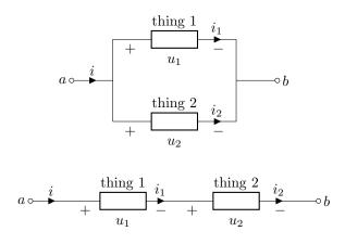
One good way of reasoning is to think what *requirement* each component puts upon the terminals of the pair of components. In this way we can try to find the u/i relation of the pair: if this matches the u/i relation of a known type of component, we can replace the branch with that component, which will be *equivalent* when seen at the terminals a and b.
