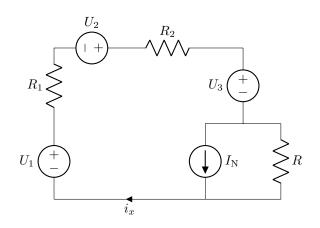
you could reduce the circuit to a single loop by transforming this Norton source to the equivalent Thevenin source of  $U_{\rm T} = RI_{\rm N}$  and R, then combine all the series components into a single voltage source and resistance,
