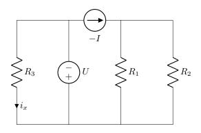
Notice how parallel branches, such as  $R_3$  and U, can be drawn in different order, or on different sides of the other components: they are still connected to the same nodes, which is all that matters.
