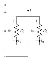
[The following should be able to be obtained by applying duality to the case of series resistors.]
