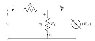
The results from the voltage divider equation will then be slightly or very wrong, depending on whether the current in this extra component is small or large compared to the current that would flow through the two resistors by themselves.
