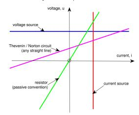
Now we can consider the dual of the above case, where we swap current with voltage, and series with parallel. We note how a current source with a *series* resistor is just like the current source: the resistor is irrelevant. But a current source with a *parallel* resistor is different: it turns out to behave similarly to a voltage source with series resistor.
