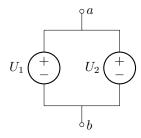
Think of what a voltage-source determines. It can have *any* current that the rest of the circuit wants. All it sets is the voltage: it rigidly requires the difference in potential (energy) between its terminals to be a set amount.
