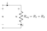
For any number of resistors all in series, the equivalent resistance is just the sum of the individual resistances. This is easy to remember, as the resistance is the difficulty of pushing a current through: if all the current has to go through one resistor then another, the difficulty is increased by each.
