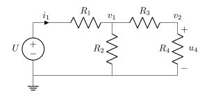
Let's suppose we need to find  $i_1$  and  $u_4$ . By the supernode method, which is generally a good way for manual calculation, we write KCL for the two nodes of unknown potentials  $v_1$  and  $v_2$ ; the other two nodes have known potentials of 0 and U.
