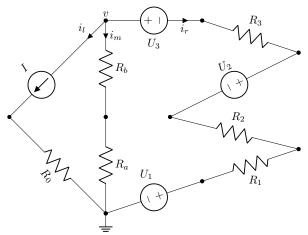
Notice that the circuit can be seen as three 'branches' between v and the ground node. If we can describe the current in each branch as a function of the known values of components and the unknown v, then a single KCL equation can be written and solved for node v.
