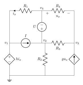
First, we note that the following necessary steps have already been made, to define the node potentials: \* Define one node as the reference potential (earth). \* Define the other nodes' potentials as  $v_1$ ,  $v_2$ , etc.
