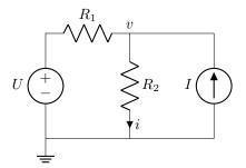
If we're going to use superposition at all, in this case with just two independent sources, there's no choice about which groups to use! One superposition state must be with just the voltage source active, and the other must be with just the current source active.
