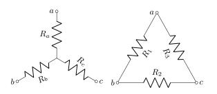
These two connections can be made equivalent, when seen from the terminals a,b,c, as long as component values fit the following conditions.
