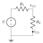
This circuit has a very easy solution for  $i_{(1)}$ , using a series equivalent and Ohm's law, or just KVL.
