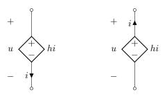
Depending on the relative direction of the current and voltage definitions, this could look like a positive or negative resistance. In the example shown at the left, the gain h is equivalent to a resistance: the relation of i and u is u = hi. By making this value negative, or by swapping the current definition as shown on the right, the component looks like a negative resistor, such that u = -hi when the current is defined into the positive side of the voltage reference direction.
