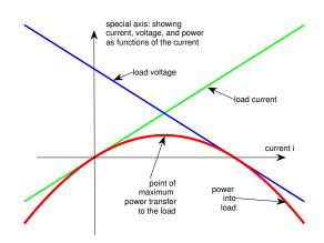
The voltage u decreases from the Thevenin equivalent's open-circuit value at i = 0, to zero when  $i = i_{sc}$ . A line showing the current i is marked as well, but this is trivial as it is just a plot of i versus  $i \dots$  its purpose is to make clearer how the *product* of the uversus i and i versus i lines gives the quadratic curve of P versus i.
