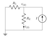
This also has a simple solution, using methods from Topic 02. Current division between the resistors gives
