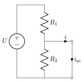
Due to the short-circuit, the lower resistor can be ignored. Its top and bottom are at the same potential, so no current passes through it. The full voltage U is across the upper resistor, and the resulting current passes between the terminals. Ohm's law provides the circuit's short-circuit current (sv: kortslutningsström),
