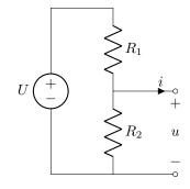
The three components, connected to two terminals shown on the right, are the circuit that we want to replace with an equivalent.
