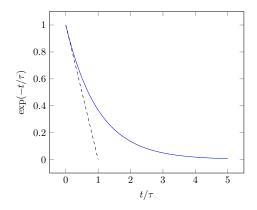
The figure (above) shows an exponential function  $e^{-t/\tau}$  at t = 0, together with its tangent (dashed) at t = 0. The tangent has a gradient of  $-\frac{1}{\tau}$ , which can be calculated from  $\frac{d}{dt}e^{-t/\tau}$  at t = 0. It therefore reaches zero at time  $t = \tau$ . In contrast, the exponential slows down more and more as it approaches its final value.
