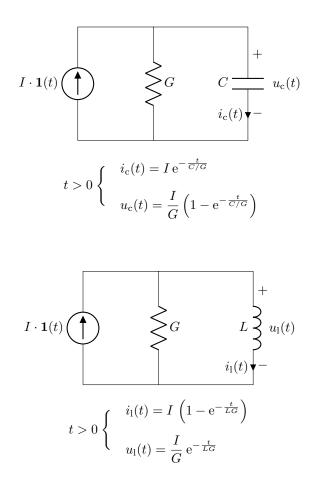
It could be educational to make a full derivation by the direct ODE method, of each of the preceding cases. One hint is to find the continuous variable, then simply differentiate that expression (and multiply by the component value C or L) to find the other variable.
