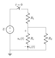
Without any reactive components, this is a static circuit, where the solution at any time depends only on the components' values at that time. So let's find what is the marked voltage  $u_c$  at any time after zero.
