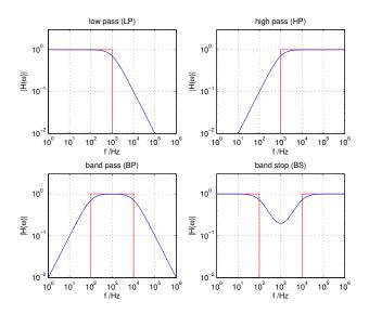
In each case the red lines show an "ideal" response, which cannot be attained in reality. The smooth blue curve shows a very simple implementation with a network function that could be made from one or a few simple circuit-elements.
