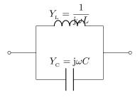
the equivalent admittance at angular frequency  $\omega$  is
