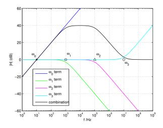
Notice that the decibel amplitudes of the separate terms have been added to find the decibel amplitude of the total network function. This may sound strange, as the separate terms are *multiplied* in the network function: it works because the decibel scale is logarithmic, and  $\log ab = \log a + \log b$ . Hence, for example, if dB(·) = 20 log<sub>10</sub>(·),
