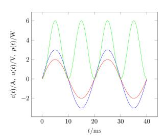
There is nothing strange about the blue and red curves of u(t) or i(t), but the curve of p(t) (green) may look surprising. It's always positive ... which is reasonable, as a resistor cannot ever produce power. It alternates, but at *twice* the frequency of the voltage or current: after a little thought, that sounds reasonable, as there is still a positive power when the voltage and current are *both* negative. The shape looks like a sinusoid but added to a constant "dc offset".
