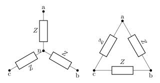
The one the left is the same as was used for the voltage sources that we looked at earlier. This type of connection can be called *star wye* (Y), based on its shape. Each terminal connects to one end of just one of the impedances. The other ends of the impedances connect together, to a point that has been labelled 'n' for neutral: this is sometimes called the *star point*.
