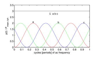
We can note how the individual phases have powers oscillating between zero and twice their mean value, but the total power input at any time is a constant of three times the mean value of each phase.
