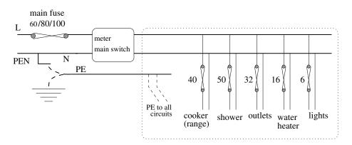
Note that a given load on a three-phase connection would need each of its three wires to carry only 1/3 of the current compared to each of the two wires if the same load power is supplied from a single phase and neutral (from a system with the same three-phase voltage). In the above diagram, many countries would have multiple 16 A circuits for socket outlets, but in the UK it's common to have one to three bigger circuits to many sockets, then to have smaller fuses in the plugs.
