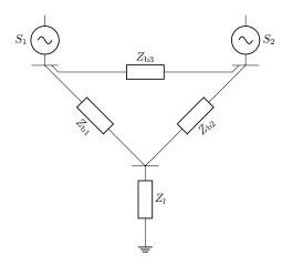
In this way, one makes calculations as if on a single-phase circuit. It's just occasionally necessary to remember that in fact the system is a three-phase one – for example, if you wonder why a meter tells you it's 230 kV to earth, whereas you were calling it a 400 kV line. By a normalization called the power system "per-unit" method, even the factor of  $\sqrt{3}$  when calculating powers is not needed.
