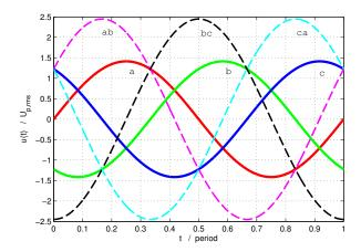
After phase-a has had, for example, a positive peak, then the phase that has its positive peak soonest afterwards is phase-b, and then phase-c. There are only two possibilities for phase-sequence: abc and acb (you could also write e.g. cba, but this is the same sequence as acb if it keeps repeating).
