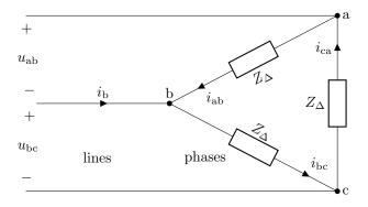
Now the situation is reversed: each phase of the load has a voltage equal to the line voltage. But each line current is a phasor sum of the two phase-currents of the impedances that connect to the line. For example,
