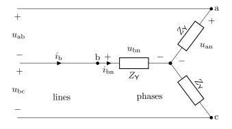
The current through each phase of the Y-connected load is clearly the same as the current in the supply line that is connected to it,
