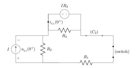
Notice that at  $t = 0^+$ , the current source I in the original circuit is short-circuited by the capacitor  $C_2$ and the closed switch. It is therefore irrelevant to the requested variables. (However, the quantity 'I' is still relevant, as this is included in the expressions for the current in inductor  $L_1$  and the voltage on capacitor  $C_1$ , still shown above.)
