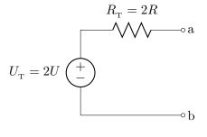
It is important to show how the terminals a-b are related to the poles of the voltage source in the Thevenin equivalent. This is conveniently done by a diagram.
