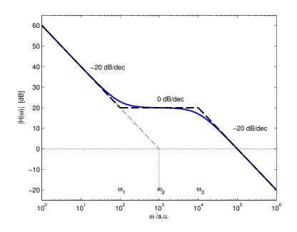
In this example the curved blue line is the actual function, without the asymptotic approximation of the Bode plot. The term  $\frac{1}{j\omega/\omega_2}$  is at 0 dB when  $\omega = \omega_2$ : the relation of  $\omega_1$  to  $\omega_2$  is what determines the level of the flat (0 dB/dec) part of the plot, because it is when  $\omega > \omega_1$  that the  $(1 + j\omega/\omega_1)$  starts to cancel the downward slope of the  $\frac{1}{j\omega/\omega_2}$  term.
