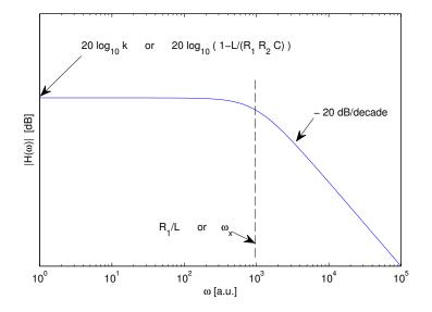
This is an unusually easy Bode amplitude plot. It is just the curve of a single pole, shifted vertically by k (in dB). The values k and  $\omega_x$  could be used, or their equivalent in terms of circuit quantities such as  $R_1/L$ . In case you wonder: 'a.u.' means 'arbitrary units'. Normally the hand-written Bode plot would use straight lines instead of showing the curve around  $\omega_x$ .
