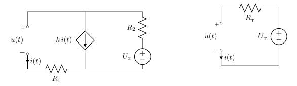
The circuit has three parallel branches. The currents in two of them are already marked as i and ki. The current in  $R_2$  can be found by KVL around the outer loop. KCL can then be written for the three currents,
