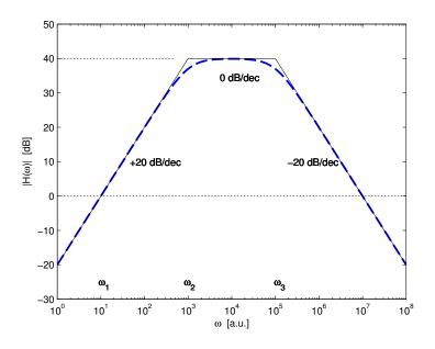
The negative sign in  $H(\omega)$  arises because of this being an inverting amplifier. It has no effect on the amplitude plot, as it changes the function's phase, not its magnitude:  $|H(\omega)| \equiv |-H(\omega)|$ .
