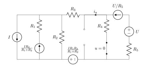
This circuit can be simplified a bit by removing some components that are irrelevant to the sought quantity of  $i_a$ , and combining components where possible. The irrelevances in this case are components in series with current sources. The combining is then possible for two parallel current sources.
