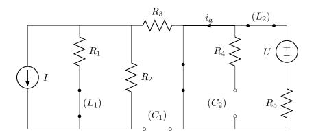
From this, we see the power delivered from source I is just the power it provides to the parallel combination of  $R_1$  and  $R_2$ ,
