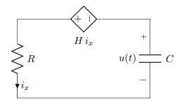
By KVL,  $Hi_x + u - Ri_x = 0$ . This has two unknowns, but as the current  $i_x$  is also the current passing upward in the capacitor, we can further include the relation of u and i in a capacitor  $(i_x = -C\frac{du}{dt})$  to get a differential equation in just u or just  $i_x$ . We'll take the standard approach of solving first for the continuous variable, which is u:
