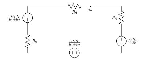
In this simplified circuit, KCL tells us that the same current  $i_a$  passes all around the loop. KVL gives an equation for the current,
