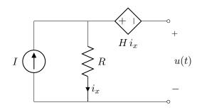
By KCL the full current I passes down through R, since the capacitor in equilibrium is open-circuit. Hence  $i_x = I$ , which determines the dependent source's value to be HI. Then KVL around the right-hand loop gives
