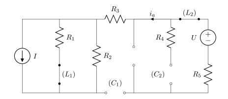
The energy in  $L_1$  depends on the current in this component:  $W_{L1} = \frac{1}{2} L_1 i_{L1}^2$ .
