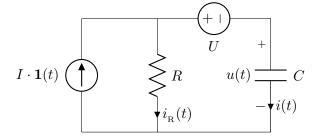
By KCL, the currents in the capacitor and resistor are related by
