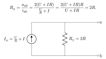
We could instead have found the Norton resistance for this circuit with no dependent sources, by simply "setting the independent sources to zero" and simplifying the resulting circuit of resistors.
