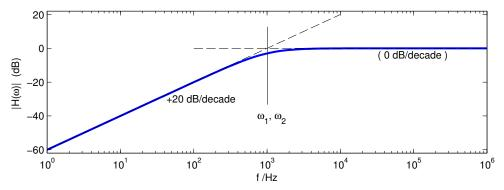
The main features to mark are the frequency  $\omega_1$  (and/or  $\omega_2$ ), the slopes (it's not essential to mark the zero slope), and the 0 dB level at  $\omega \gg \omega_1$ . As long as these details are marked, the numeric scales are not necessary: the frequency is arbitrarily chosen here. The classic asymptotic Bode plot shows straight lines, but it would be acceptable to show either the straight-line approximation or the actual, curved transition between the asymptotes.
