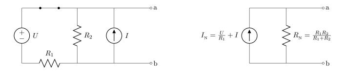
The above results can be seen by considering open-circuit conditions (in part a) or short-circuit conditions (in part b) to obtain the equivalent source values  $U_{\rm T}$  and  $I_{\rm N}$  respectively; the equivalent resistances are found by setting the (independent) sources to zero and simplifying the resulting resistor-network.
