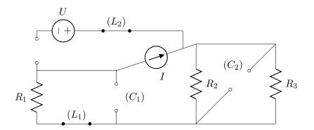
The power supplied from the current source is found by multiplying its current I by the voltage it, choosing suitable directions or signs so that the power out from the source into the circuit is found. Only
