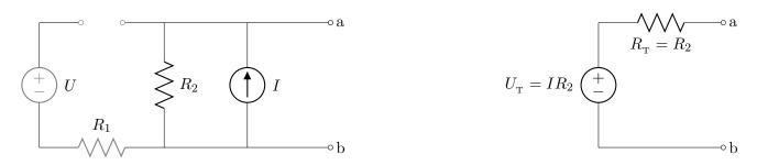
**b)** At t > 0, the circuit (left) its and Norton equivalent (right) are:
