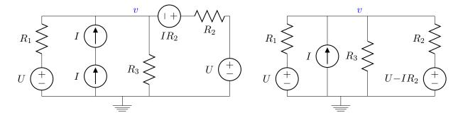
(This simplification of current sources is one of many 'theorems' for circuits. It is an example of the current-source version of Blakesley's source-shift theorem from 1894, which focused on voltage sources, http://iopscience.iop.org/1478-7814/13/1/307)
