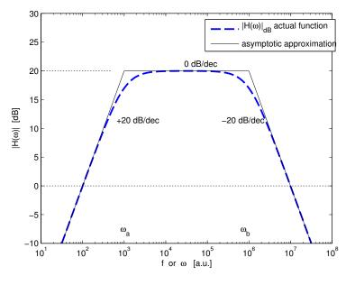
The Bode magnitude diagram can be worked out from the function itself, considering approximations when the frequency is at, or is much above or below, the special frequencies  $\omega_a$  and  $\omega_b$ .
