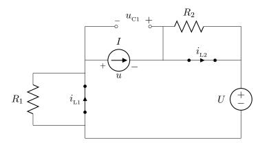
The energy stored in the capacitor is  $\frac{1}{2}C_1u_{C1}^2$ . By KVL around the inductors (short-circuit) and voltage source, this is  $u_{C1}(0^-) = U$ . So  $W_{C1} = \frac{1}{2}C_1U^2$ .
