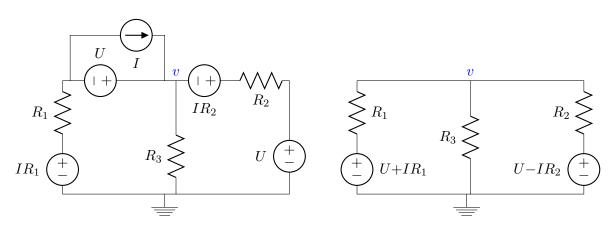
Source transformation and simplify current-sources. A quite similar simplification can be done using just one source transformation, if one realises that node 'a' in the original circuit has current sources putting equal currents in *and* out; their total current is therefore zero, so they do not affect the node. These sources can then be separated as shown below, and simplified into one.
