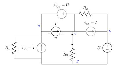
Nodal analysis. One way to solve the circuit to find the voltage across  $R_3$ , is nodal analysis without any further simplifications. The four nodes have been marked with letters. Let's define node g as the reference (ground). Then the voltage across  $R_3$  is v.
