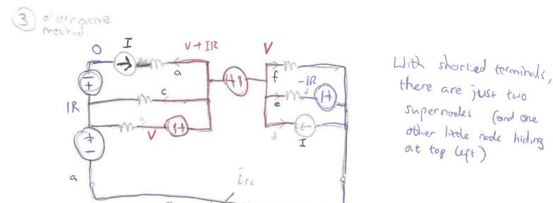
Q One nodal approach: KCL non-graind supernode: find short circuit current;  $-I + \frac{V - |R|}{R} + \frac{V + |R| - |R|}{R} + I + \frac{V - (-|R|)}{R} + \frac{V}{R}$ 0= · Short the terminals (9) (2) D 0 · Set something as zero identify sugarnodes
