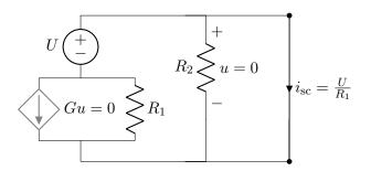
Thus, the short-circuit current is  $i_{sc} = U/R_1$ , based on taking KVL around  $R_1$ , U and the short-circuit.
