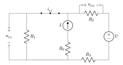
Now that we know the voltage  $u_{C1}$ , we can use KVL to show that this is also across  $R_1$ , then Ohm's law to find the current in  $R_1$ , then KCL to show that this is the current in the inductor. The result is
