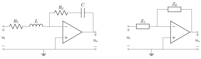
$H(\omega)$  can be found from KCL at the inverting input, where the potential must be 0 in order to match the non-inverting input:  $\frac{0-u_i}{Z_1} + \frac{0-u_o}{Z_2} + 0 = 0.$ Alternatively, one can make direct use of the standard result for an inverting amplifier,  $u_o/u_i = -Z_2/Z_1$ .
