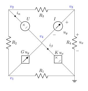
The above are 8 equations in 8 unknowns:  $v_1$ ,  $v_2$ ,  $v_3$ ,  $v_4$ ,  $i_{\alpha}$ ,  $i_{\beta}$ ,  $u_x$ ,  $u_y$ . Having followed the rules, we expect them to be independent equations.
