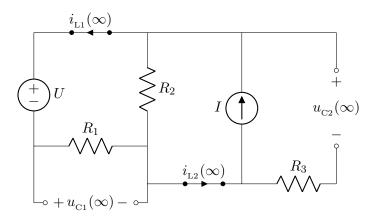
Consider first the initial condition. The capacitor's continuous quantity is voltage. We find the voltage on the capacitor in the equilibrium at  $t = 0^-$ , before the switch closes.
