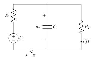
By continuity, the capacitor's voltage remains the same immediately after the circuit changes, so  $u_{\rm c}(0^+) = u_{\rm c}(0^-) = \frac{UR_2}{R_1+R_2}$ .
