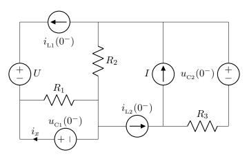
The power out of  $C_1$  is  $u_{C_1} i_x$ , where  $i_x$  is the current shown above, defined out of the + terminal of the voltage source that represents  $C_1$  at  $t = 0^+$ .
