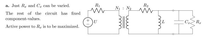
This is a very classic ac maximum power case. With  $R_x$  and  $C_x$  forming the load, we can freely control both the active and reactive parts of the load, and the reactive part of the load is the opposite type to the source. It is therefore possible to fulfil the maximum power condition  $Z_{\text{load,maxP}} = Z_{\text{source}}^*$ .
