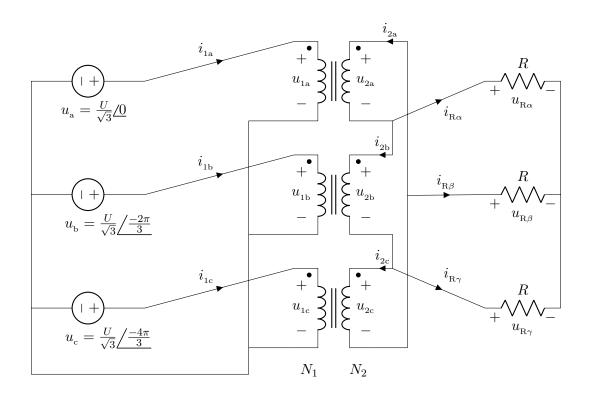
Note that straight lines crossing each other in this diagram do *not* indicate a connection. Connections here involve three lines stopping at a single point.
