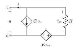
Here, writing a relation between u and i looks a good idea. The presence of dependent sources prevents the method of just simplifying resistors after setting all independent sources to zero.
