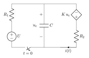
In the initial equilibrium at  $t = 0^-$ , with the switch closed and no current in the capacitor, we can take KCL at the top node,
