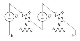
However, it's easier to take just one of the two identical parts in the circuit. If we define the middle point at 0 and define a current *i* out of terminal 'a', KCL gives  $i + \frac{v_a}{R} + \frac{v_a - U}{R}$ , from which  $v_a = U/2 + i R/2$ . We get the solution by identifying  $U_{\rm T}$  and  $R_{\rm T}$  from this u, i relation, and doubling them for the case of two similar series-connected units.
