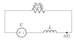
**b.** The power into the inductor is the product of its current and voltage, with suitable choice of sign. If we define the inductor's voltage as u with its reference side (+) where the current i goes in, then from the relation of inductor current and voltage,
