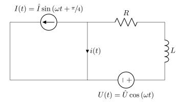
Start by defining the circuit as phasors and impedances instead of time functions.
