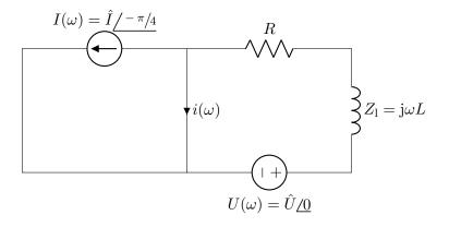
The marked current i can be found by KCL from the currents in the left and right branches.
