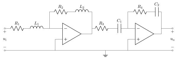
The input to the second amplifier (the left side of  $R_3$ ) connects to the first amplifier's opamp output. This is a stiff voltage source, which the left opamp forces to be whatever potential is needed to ensure that its inverting input stays at its inverting input's zero potential. So this is not affected by whatever current flows through  $R_3$ . The two amplifiers can therefore be analysed separately, and their network functions combined to give the total network function.
