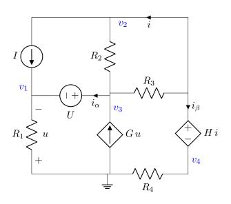
$$\text{KCL}(1)_{(\text{out})}: \quad 0 = \frac{v_1}{R_1} - i_\alpha - I$$
