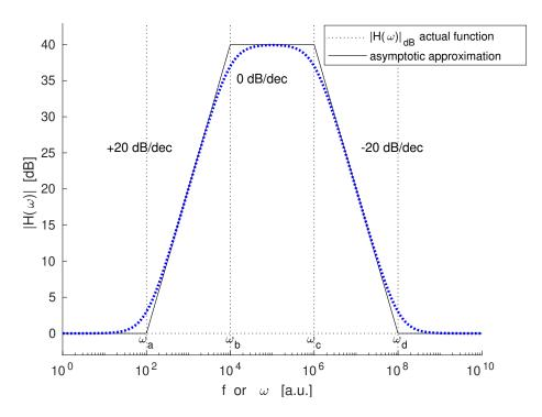
Necessary parts are: the asymptotic approximation lines, the gradients of the up and down slopes, the 0 dB and 40 dB levels, and the locations of  $\omega_{a,b,c,d}$ . The actual curve is not needed. The flat parts do not need marking with 0 dB/decade. No numeric frequencies are needed.
