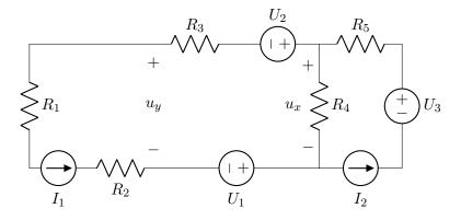
Source  $I_2$  with KCL already determines the current up through  $U_3$ . Source  $U_3$  determines its own voltage. The product of voltage with current out of the voltage's + terminal ('active convention') is the power out of the component.
