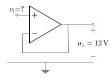
(A thought: Does it make sense to talk of a potential [which means relative to the shown earth] or to mark a voltage  $u_0$ , in spite of the upper part of the circuit showing no component or node connecting to the earthed node at the bottom? These could seem like two separate 'circuits'. But remember: an opamp symbol hides some details!)
