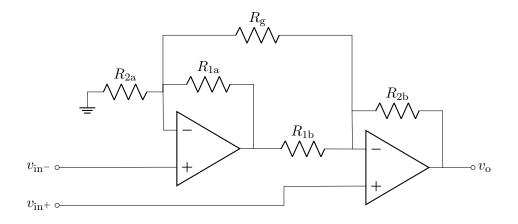
Assume  $R_{1a} = R_{1b} = R_1$ , and  $R_{2a} = R_{2b} = R_2$ .
