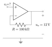
a) This is a buffer. Its output follows the input. This can be inferred from the assumption that, given negative feedback and an ideal opamp, the two input potentials are equal,  $v_{+} = v_{-}$ .
