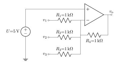
The output potential includes a sum of the input potentials and a constant. This is multiplied by a (negative) gain. So the circuit is an inverting amplifier with multiple inputs. Its output depends on the "weighted sum" of the inputs (with the equal resistors shown in the example, the weights are equal).
