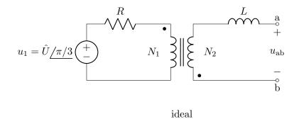
a) Find the Thevenin equivalent of this circuit, seen between the terminals a and b.
