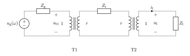
This is a good (simple) model of how most of our electric power gets to us: it is generated at one voltage, then "stepped up" to a higher voltage for transmission, then "stepped down" to a low voltage for final use.
