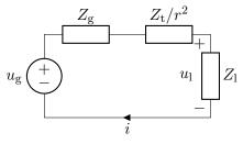
**d)** Let  $|u_g| = 50 \text{ kV}$ , and r = 2. Use the voltage  $u_g$  as the phase reference (zero). What are the voltage, current and complex power at the load:  $u_1$ ,  $i_1$  and  $S_1$ ?
