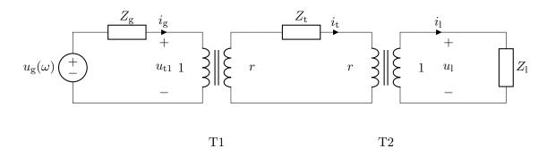
This is a good (simple) model of how most of our electric power gets to us: it is generated at one voltage, then "stepped up" to a higher voltage for transmission, then "stepped down" to a low voltage for final use.
