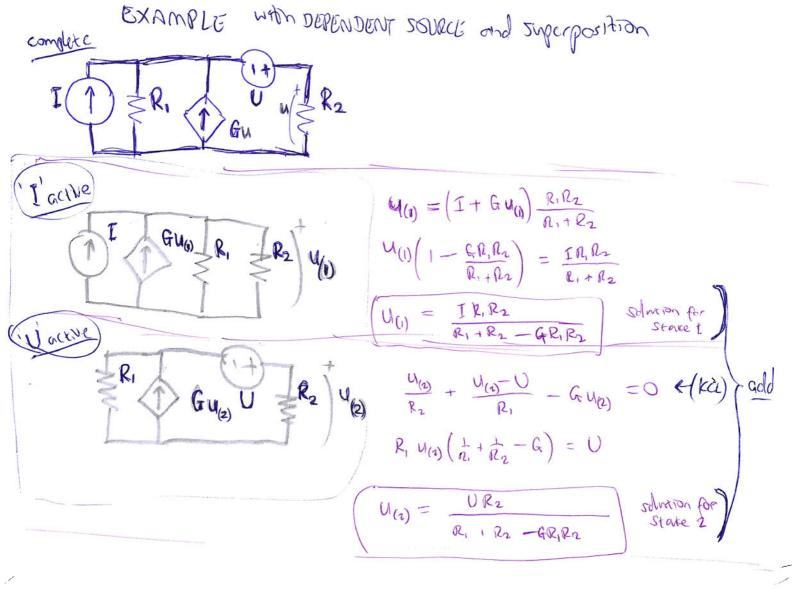
(ontinued)  $U = U_{(1)} + U_{(2)} = (U + IR_1) R$ R, + R2 - GR, R2 That might seem necut But in this case, nodal analysis (KCL) on the Whole circuit including both sources would probably have been independent Just add a "-I" term in the starte(2) solution on the previous page.) equicker and easier ... try A!
