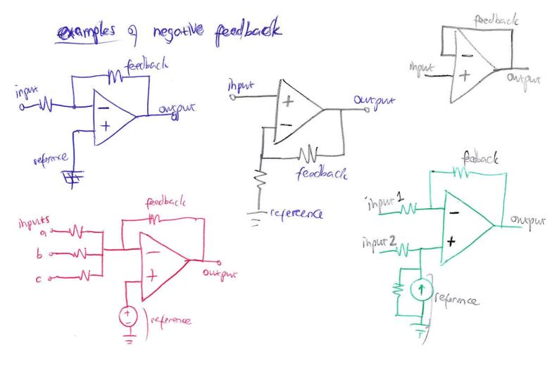
Summary of "rules" for openp circuit solution - $\begin{bmatrix} negative feedback \\ and \\ infinite sain \\ \end{bmatrix} \xrightarrow{Can}_{assume} V_{+} = V_{-}$ finfinite input resistance no current into inputs Output is like udtage source (getting its current from earth node) ) output current is determined by what's connected ... voltage is whatever the feedback needs in order to ensure that V=V+ THIS, WITH (KCL, KVL, Ohn ? is all you need opamp circuits can be solved using these rules
