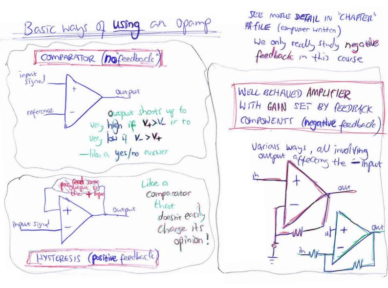
NEGATIVE FEDBRACK - the way of taming a wild high-gain amplyier into a controlled amplyier of chosen gain. hput Signal may go to autput D of O or botch - negative feedback, males the Output affect the inverting reference Signal ihput by some controlled propertion esg if V+>V, autput goes up so it helps V- go up, so the difference 4-V. is reduced. Infinite frain AND Negotile readback - 4=4
