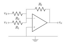
The output voltage is whatever is needed to allow all this input current to flow through the feedback resistor  $R_{\rm f}$ .
