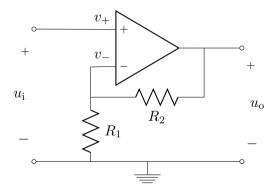
That means the output has to 'work harder' to force  $v_{-} = v_{+}$ . If we divide by 10, the output must become 10 times as much as the input!
