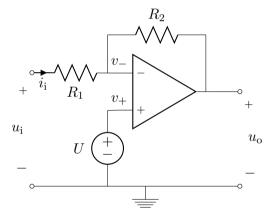
The source introduces constants in the equations for e.g.  $u_0$  and  $i_{\text{in}}$ . Then it **cannot** be assumed that  $\frac{\Delta u_0}{\Delta u_i} = \frac{u_0}{u_i}$ .
