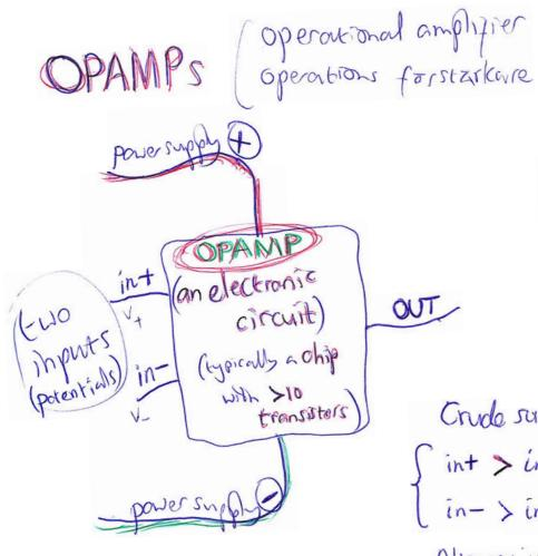
Not a fundamental "component for modelling basic physics like a wire, battery, etc But very Versatile and widely used. so we should know about it.
