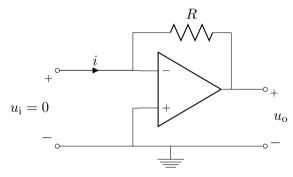
Here, the input is held to a constant 0 V (virtual ground) by the feedback.
