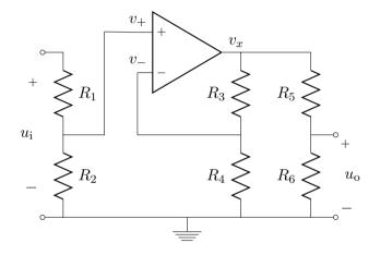
In the earlier circuits we didn't discuss *output* resistance. In fact, those amplifiers' outputs behaved as ideal voltage sources, driven directly by the ideal opamp output:  $R_{\rm o} = 0$ .
