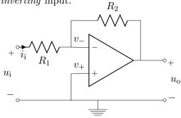
By negative feedback and ideal opamp behaviour, the opamp's output adjusts to be whatever is needed to obtain  $v_{-} = v_{+}$ .
