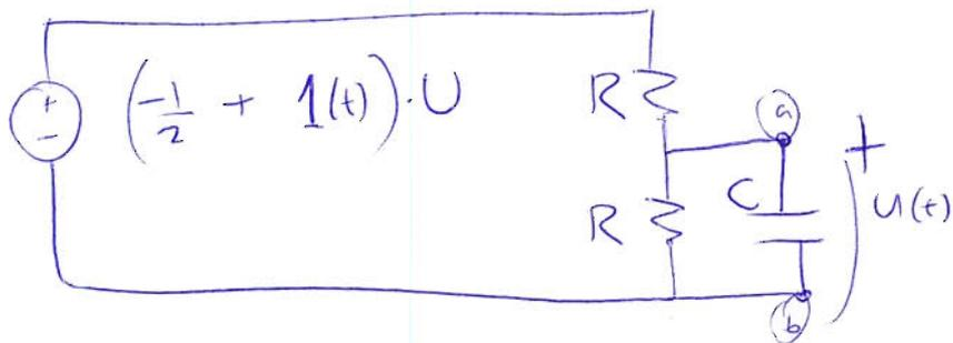
By considering how the Thevenin equivalent has changed at terminals a-b by adding the extra resistor, find the new function of  $U(t)$ .
