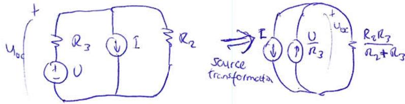
$$U_{oc} = U_T = \frac{\left(\frac{U}{R_3} - I\right) R_2 R_3}{R_2 + R_3} = \frac{UR_2 - IR_2 R_3}{R_2 + R_3}$$
