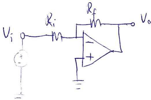
$$V_o = -\frac{R_f}{R_i} V_i \quad \Rightarrow \quad \frac{V_o}{V_i} = \left( -\frac{R_f}{R_i} \right)$$
