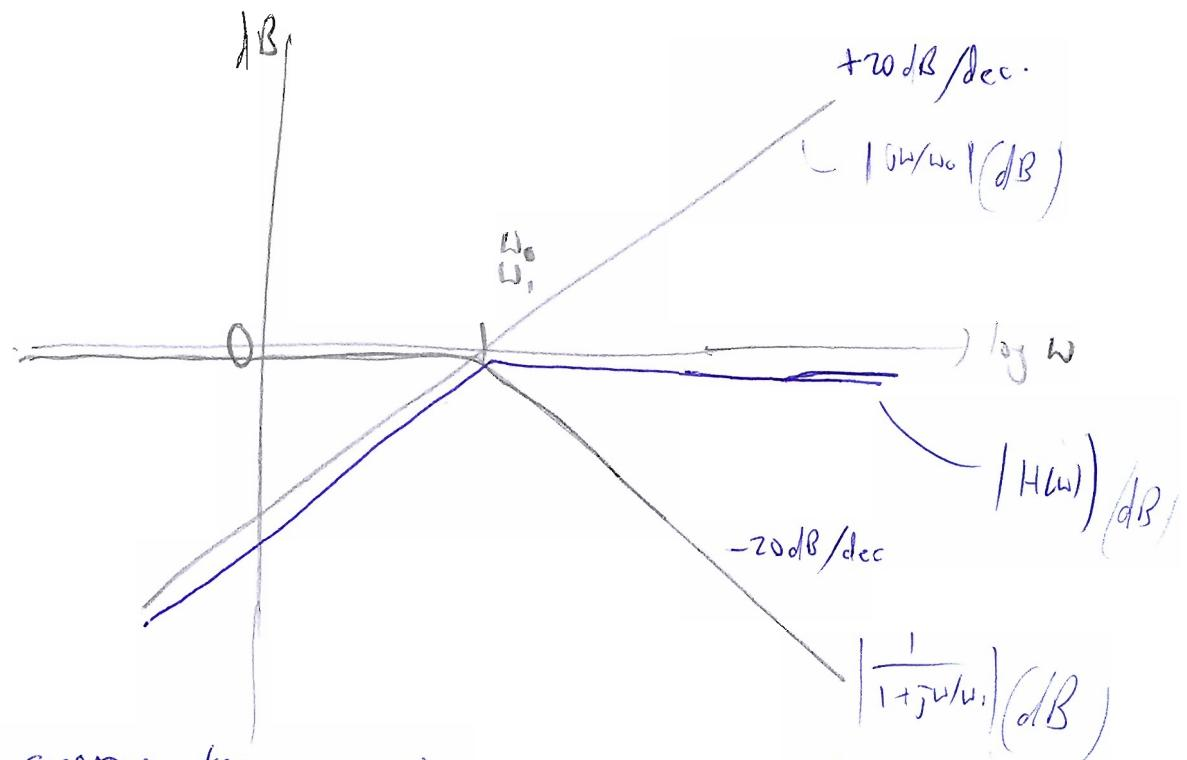
The separate terms are the same as before, but shifted horizontally to fit  $\omega_0 = \omega$ . The result is a similar shape to the previous case, but shifted downwards.
