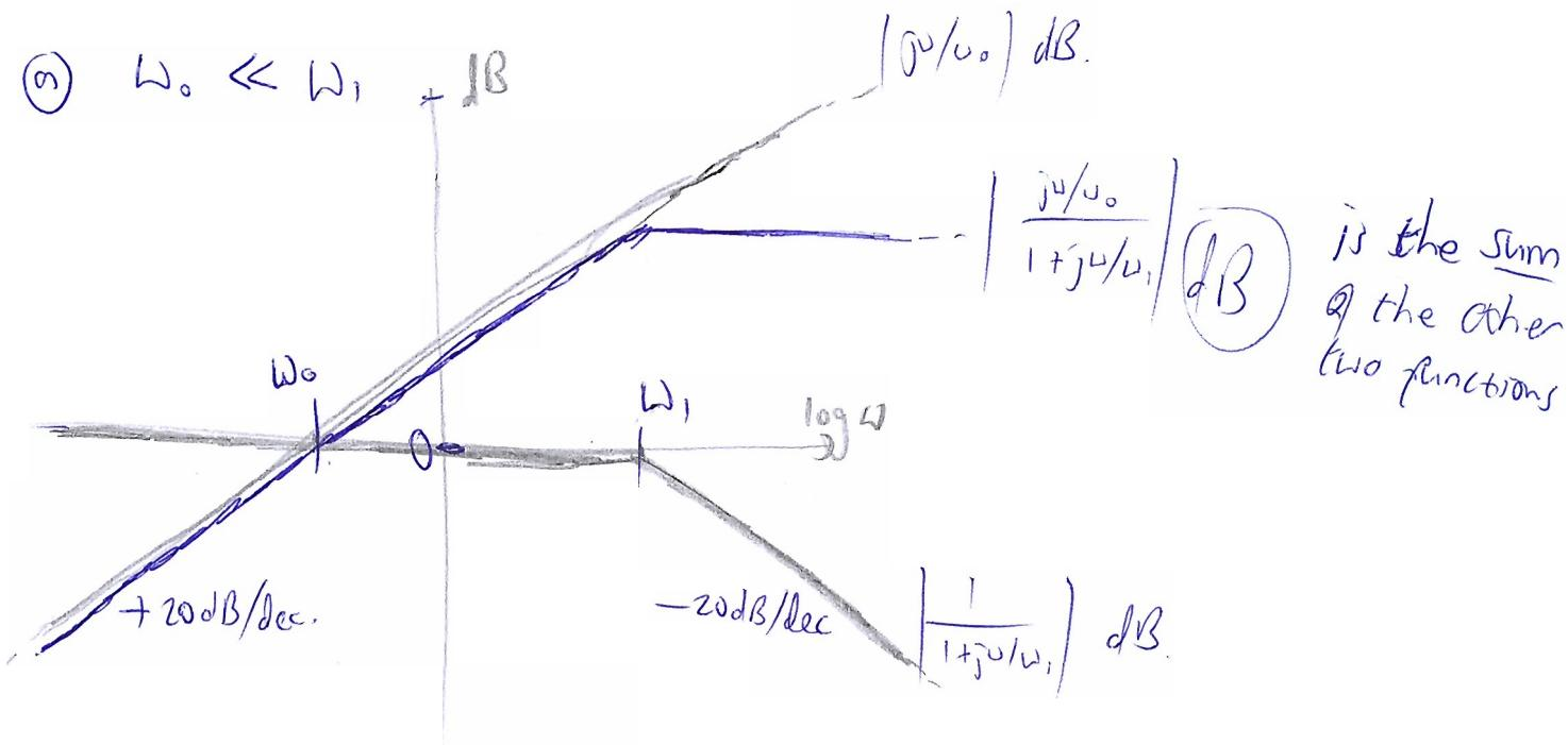
In this region the total is the sum of 0dB (constant) and the  $+20 \text{ dB/dec}$  line passing through  $\omega_0$
