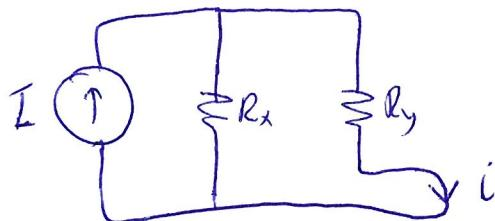
$$i = \frac{R_x}{R_x + R_y} I \quad \Rightarrow \quad \frac{i}{I} = \frac{R_x}{R_x + R_y}$$
