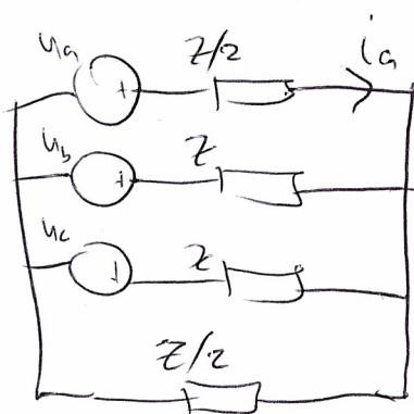
By the "Thevenin + balanced-system" method, we see easily that  $U_T$  is unchanged and  $Z_T$  becomes  $Z/5$  instead of  $Z/3$ . as the neutral adds in parallel.
