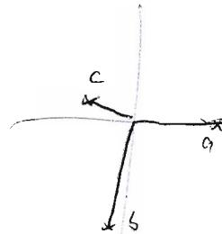
{ line or load has different impedances in phases
