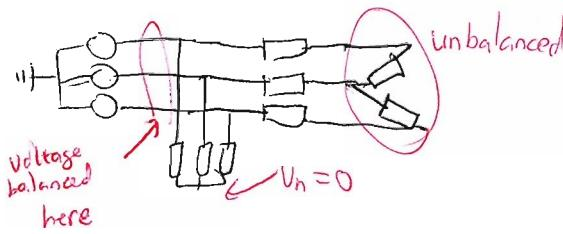
In these systems the unbalance only affects the voltage on the right of the line impedance.
