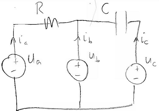
$U_{a,b,c}$  are a balanced 3phase source with line voltage  $\sqrt{3}U$  and phase rotation abc
