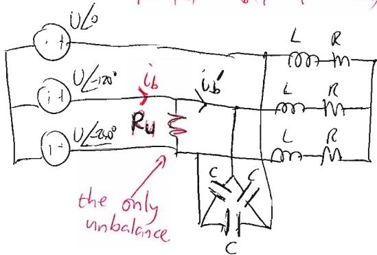
The unbalanced part is connected to an ideal voltage source. So it doesn't affect the voltage applied to the other loads. We can do balanced calculation for  $i'_b$  then add (as phaser) the current through  $R_u$ .
