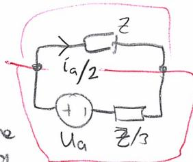
$$\frac{i_a}{2} = \frac{U_a}{Z + Z/3} \quad \therefore i_a = \frac{2U_a}{\frac{4}{3}Z} = \frac{3U_a}{2Z} = \frac{3U}{2Z}$$
