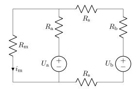
With  $U_{\rm a}$  active and  $U_{\rm b}$  zeroed (short-circuit) some combination of current and/or voltage division helps us. Let's call the three series resistors  $R_3 = R_{\rm b} + 2R_{\rm s}$ . The following circuit will still give the same solution of  $i_{\rm m}$ .
