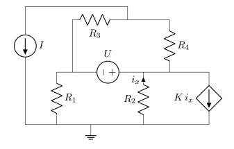
For simplicity of equations, the question defined that all of the resistances are R, i.e.  $R_1 = R_2 = R_3 = R_4 = R$ . We'll start by using the unique names such as  $R_1$ , to make clear which component is meant: then we'll change these to R when simplifying.
