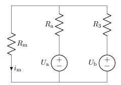
State (1): With  $U_a$  active and  $U_b = 0$ , we get the following circuit, which is simplified on the right by redrawing.
