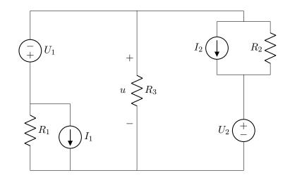
Find *u*. Values:  $U_1 = 6$  V,  $U_2 = 3$  V,  $I_1 = 2$  A,  $I_2 = 4$  A,  $R_1 = 24 \Omega$ ,  $R_2 = 24 \Omega$ ,  $R_3 = 12 \Omega$ .
