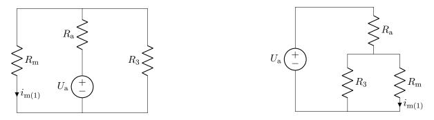
The current through  $R_a$  is found by Ohm's law on the total resistance of the three resistors. Current division lets us find  $i_m$  from this:
