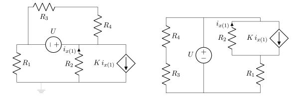
From this re-drawing, we see that the resistors on the left don't affect the solution of  $i_{x(1)}$ : the voltage source is connected in parallel with this pair of resistors, so we can reduce all of U,  $R_3$ ,  $R_4$  to just the source U without affecting the branch where  $i_{x(1)}$  is marked. To put it another way, we can write KVL around the loop U,  $R_1$ ,  $R_2$ , without being affected by the components on the left.
