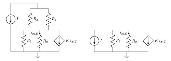
The potential of the top node can be expressed as  $-i_{x(2)}R_2$ . By KCL,
