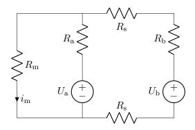
What value of  $R_{\rm m}$  (as a function of U and R) will result in the highest possible power being delivered to  $R_{\rm m}$ ?
